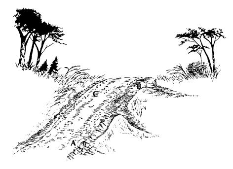
Figure No. 5 Water Turnout Construction
